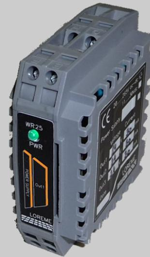
The WR25 is a DC-DC converter suitable for harsh industrial environment. Provide a perfect load separation (low input/output capacity), embed a high efficiency EMC filter. Useful for decoupling of sensitive equipments and for elimination of ground loops.
